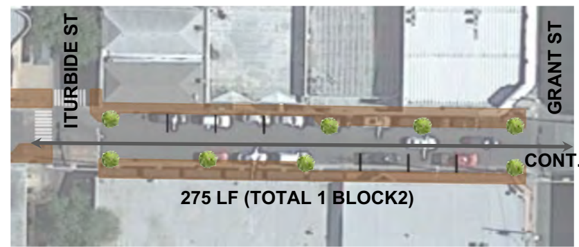
ITURBIDE ST. TO GRANT ST. IMPROVEMENTS: SIDEWALKS, LIGHTING, TREES, PARALLEL PARKING. (PRIORITY #1 – TO BE PROVIDED BY TxDOT TASA PROGRAM)
